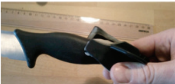
Fig. 6 - developer testing Mockup 2 gripper placement on kitchen knife
